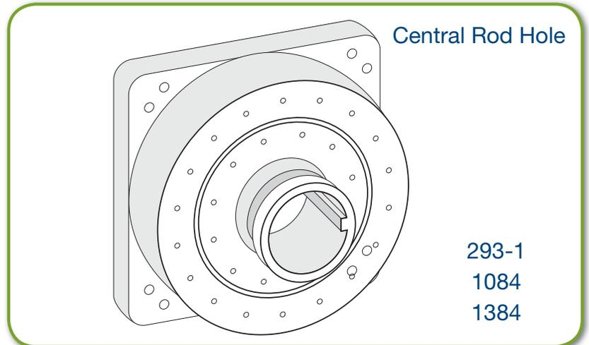
This disposable prostate template is made of Medical Grade Silicone Elastomer. The hole pattern is as shown in the figure.
