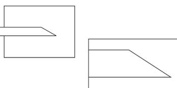
The Implant Needles are made of Stainless Steel and are hollow with different types of bevel at one end. Various lengths in different gauges are available, though the most commonly used needle is the 17G. Different types of Implant Needles are listed below:
