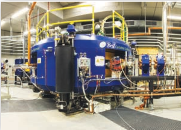
Installation of Best TM 70 MeV Cyclotron at INFN, Legnaro, Italy
