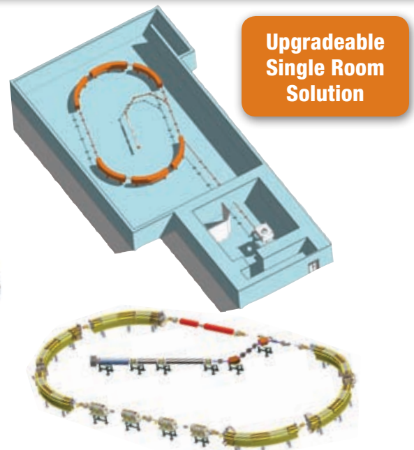
ion Rapid Cycling Medical Synchrotron (iRCMS) Racetrack
