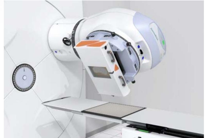
Multi-Leaf Collimators now available as an optional accessory for the Equinox and GammaBeam 100-80 product line, providing 3D Conformal Radiation Therapy (3D CRT) and Intensity Modulated Radiation Therapy (IMRT) capability.
