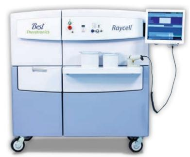
The Raycell Mk2 model features a larger chamber for irradiation of more blood bags (fits 2.0 L, 3.5 L or 6 canister model), for those facilities with higher volume needs.
