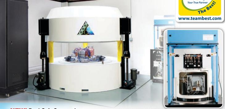
**NEW!** Best Sub-Compact Model 200 Self-Shielded Cyclotron with Optional Second Chemistry Module (Patent Pending)
